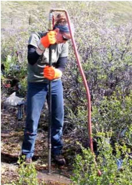
Student Kyla Smith water-jet drilling through permafrost in glacio-lacustrine sediments, Wolf Creek, Yukon
